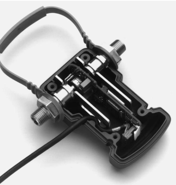
Figure 2. 700 Series Pressure Modules are overmolded with protective urethane and sealed against dirt, dust and moisture. All fittings are made of 316 stainless steel or Hastelloy C276 and have internal mechanical supports
